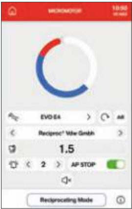
Reciprocating mode. A combination of reciprocating mode (i.e. alternating rotation movement) and the EVO E4 contra angle allows use of RECIPROC®, RECIPROC BLUE® and WAVEONE GOLD® endocanal files. The endodontic file identification trademarks are not owned by Cefla or any of its associated companies.
