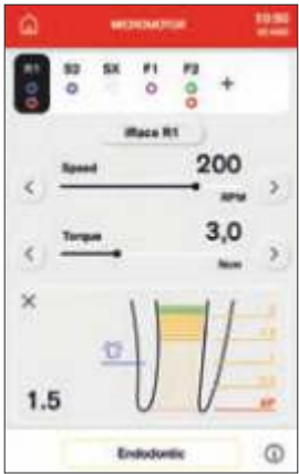
Apex locator. The apex distance is indicated on the display during the root canal instrumentation phase. The nearing of the apex is verified by the ENDO software. Once the apex is reached the Apex-Stop function interrupts micromotor rotation.
